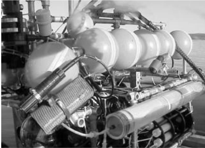
*Figure 2. Remotely operated vehicle from Eastern Oceanics used to collect vent and bottom water.*
