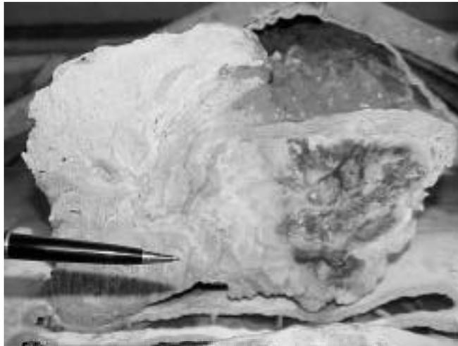
*Figure 9. Cross-section of the spire viewed from the bottom reveals the porous sinter on the left and the harder main spire with dark precipitates to the right. Pen segment is 3 inches long. (Russell Cuhel)*
