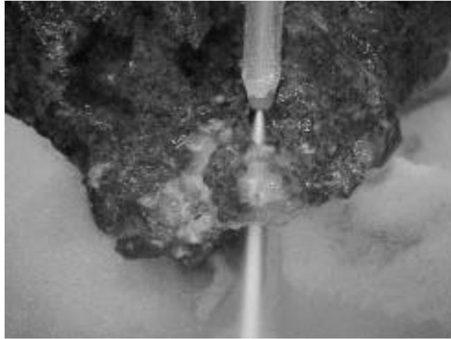
*Figure 12. No sample disintegration occurred even as the cut approached the thin, delicate tip of the main spire segment. (Russell Cuhel)*
