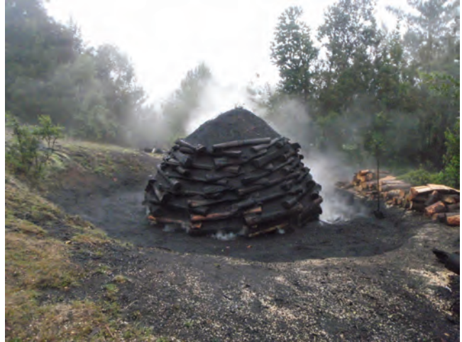
Figure 3. Photo of the home-made, earthen oven used for the production of charcoal.
