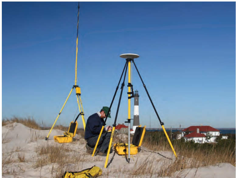
Figure 4. Field site showing geodetic-grade GPS base station. (Photo credit: Cheryl Hapke, USGS).
