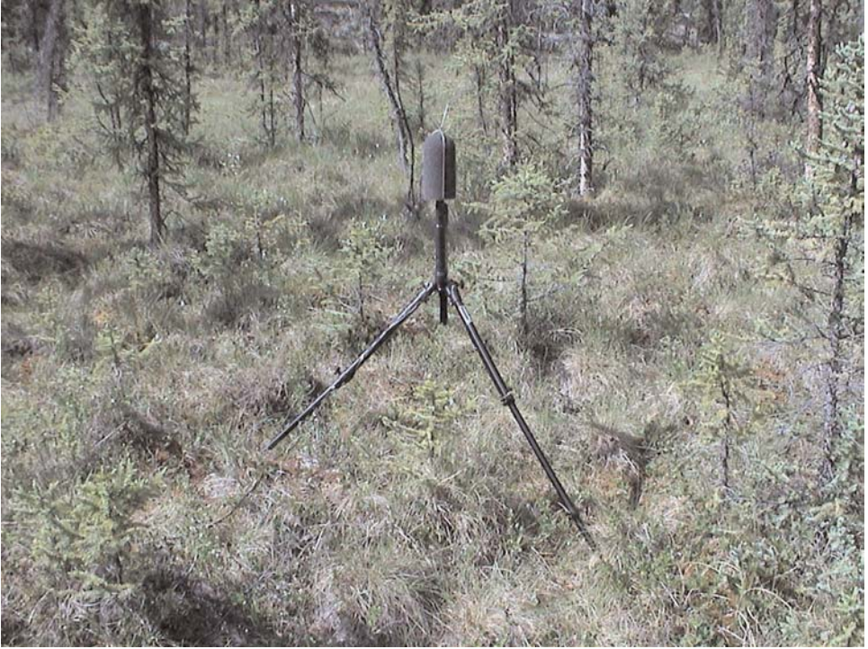
Figure 3. Microphone with foam wind screen and bird spike set up in Yukon–Charley Rivers National Preserve, 2002. National Park Service photo.
