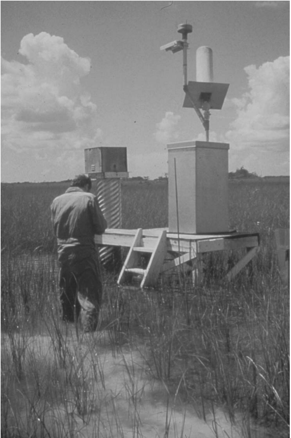
Figure 1. Environmental monitoring, such as collecting hydrology and weather data, is part of the management routine at Everglades National Park, Florida. National Park Service photo.
