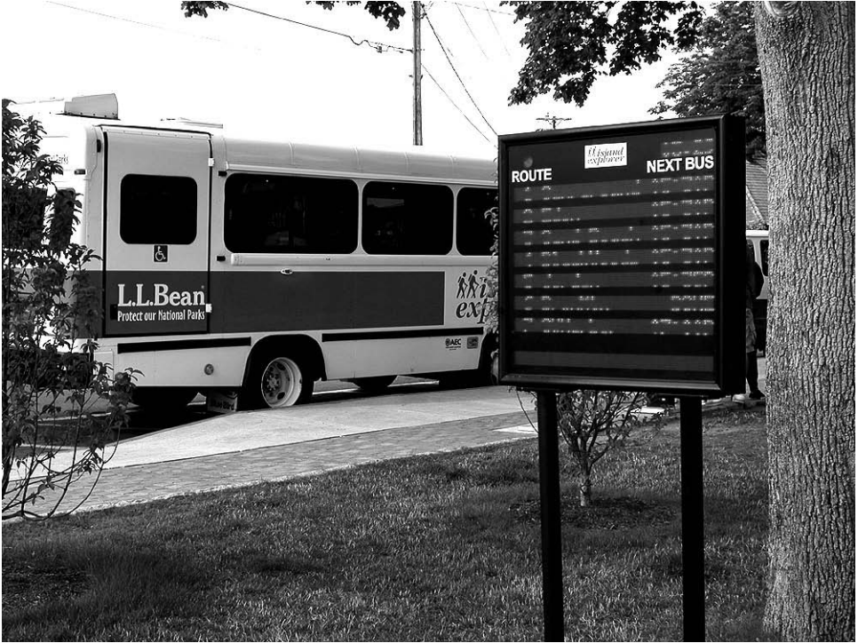
Figure 3. Acadia National Park was selected by the U.S. Departments of Transportation and Interior to test the effectiveness of intelligent transportation systems (ITS) in dealing with transportation problems within a national park setting. Real-time travel information was collected and disseminated to visitors on Island Explorer buses via an automated annunciator that transmitted an audio message and displayed the next bus stop on an electric sign within the bus. In addition, electric signs displayed real-time departure times of the next Island Explorer bus at bus stops. Pictured here is an electric bus departure sign at Village Green, Bar Harbor, Maine.
