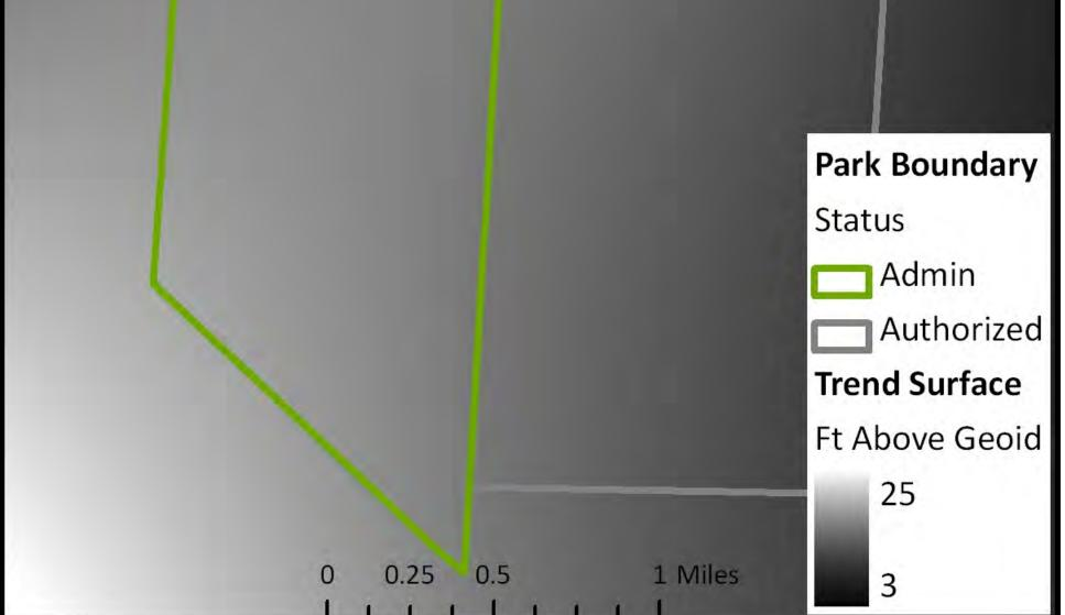
From a resampled 80ft BE model, a 3<sup>rd</sup> order trend surface was created. Both lesser and greater point densities were tested, but this density eased processing demands and effectively represented the surface for trend analysis. The 3<sup>rd</sup> order level of fit worked best, as lesser orders over-generalized, and higher orders did not adequately separate 'departures from trend'.
